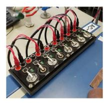
Small coin cell batteries are tested, showing that a novel UA polymer can increase battery energy density
